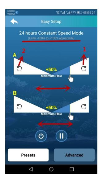
10. No matter on which preset, you could click the below buttons (1) to turn off Gyre controller, (2)To start the feed mode. While in feed mode, after the feed time is set, it will start counting down immediately.
