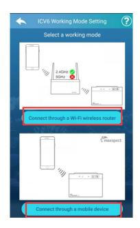
4. Select the working mode, and follow the instructions on apps to add an ICV6. In this case we screen shot on how to "Connect the ICV6 through a mobile device"
