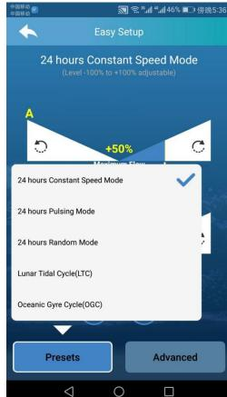
9. For different presets, the adjustable range for the parameter is different, which is also written on the headline. The rotating direction is also marked on the page, as shown in below picture, (1) is Forward Rotating; (2) is Reversal Rotating.
