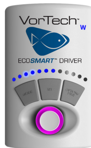
Illustration above shows an EcoSmart Driver in EcoSmart Mode (Purple Control Dial). The third and fourth brightly illuminated LEDs show that this driver is set to EcoSmart NTM along with the dim LEDs showing the speed setting.
